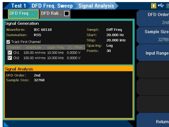
Figure 7-42 DFD Frequency Sweep > Signal Analysis settings menu page
